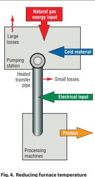
Fig. 4. Reducing furnace temperature and adding a heated transfer pipe saves significant energy due to the reduced heat flux from the large surface area of the furnace
