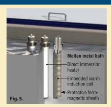
yielding a very uniform temperature profile and leaving none of the target areas susceptible to freezing.
